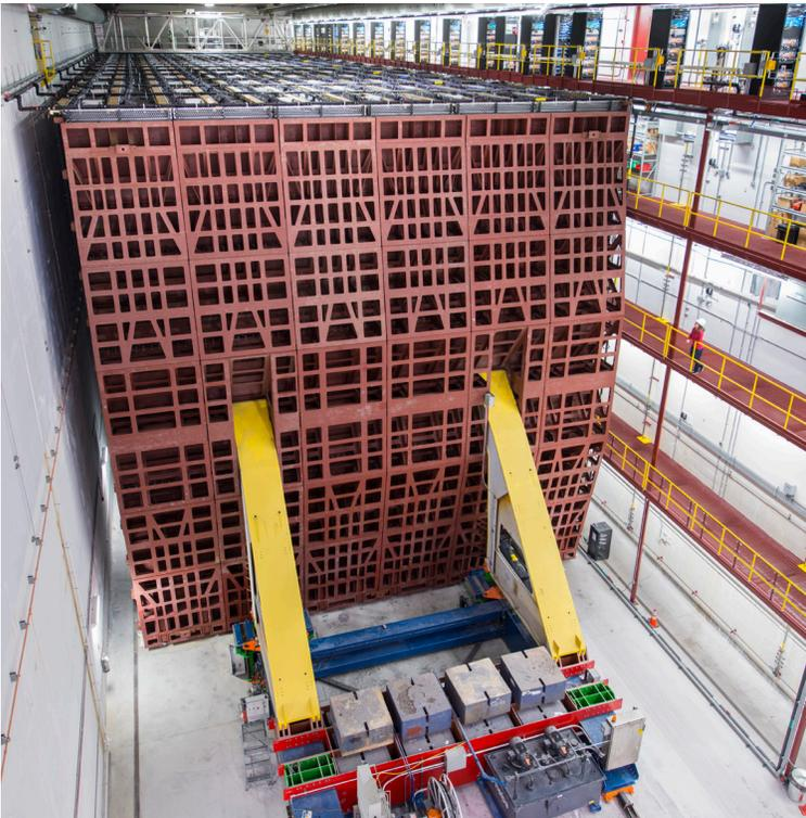
The NOvA detector in Minnesota occupies an area about the size of two basketball courts. It is 200 feet long and made of modules 50 feet high and 50 feet wide. The detector records particle tracks from neutrinos sent by a powerful accelerator at Fermilab. The construction of the NOvA detectors was completed in the fall of 2014, on time and under budget. The experiment is scheduled to collect information for six years.
