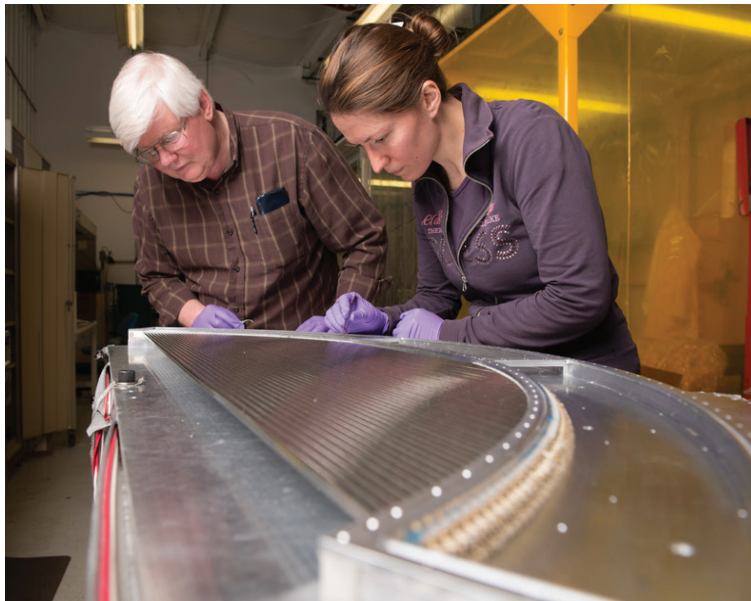
Inside Mu2e’s particle detector, about 23,000 metalized-Mylar straws are arranged in panels and filled with gas to record particle tracks.
