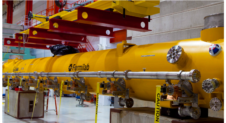
One of the first SRF cryomodules designed, built and tested at Fermilab.
