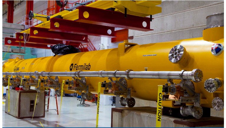
One of the first SRF cryomodules designed, built and tested at Fermilab.
