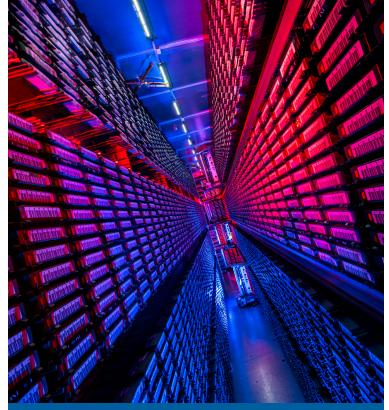
Seven commercial tape robotic systems provide more than 500 petabytes of storage capability at Fermilab. One of the largest systems available today, it could store about 3,500 years worth of full HD-quality movies. Fermilab is embarking on a new facility to host scientific data for a wide range of disciplines.
