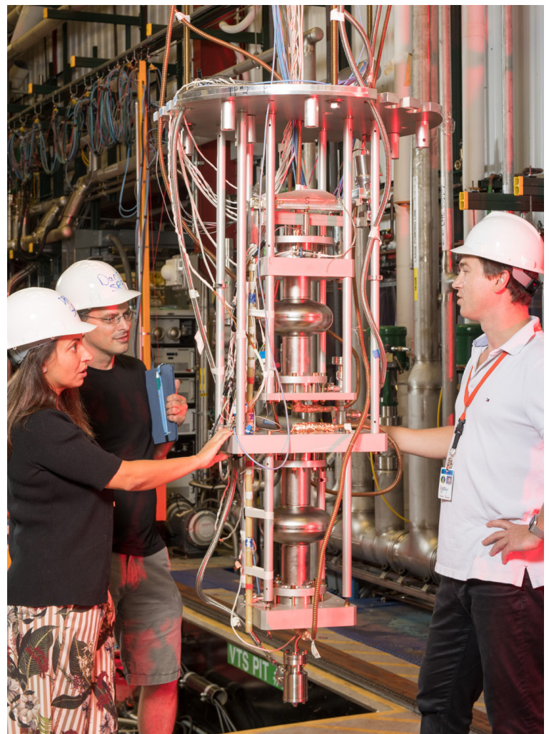
At the SQMS Center at Fermilab, scientists will leverage superconducting cavities to extend qubit coherence times. Photo: Fermilab
