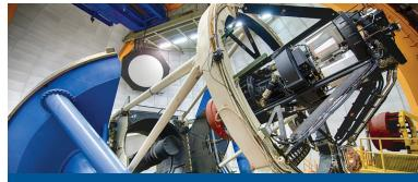
The Dark Energy Camera is mounted on NSF's 4-meter Blanco Telescope at the Cerro Tololo Inter-American Observatory in Chile.
